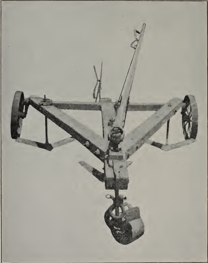
Fig. 12.—An efficient 4-horse weeder used for many years in morning glory control. This three-blade type is best adapted to rough land.
